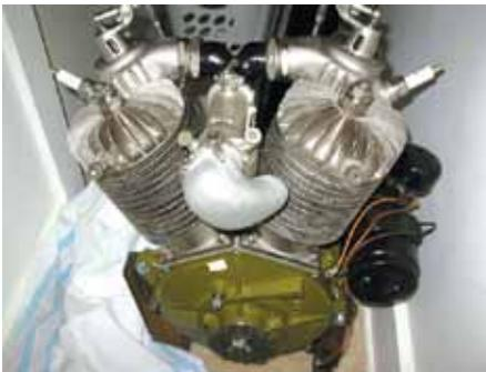
featured intake-over-exhaust valve configuration. In 1937, that engine was redesigned to include a recirculating lubrication system, and designated the model U, and it went into the same frame and running gear configuration as the model E Knucklehead, which had
